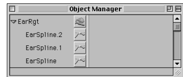
10 ... After dropping the ear splines in the EarRgt object, ensure that they are listed in this order. The order of the splines is critical—the surface is stretched over the splines in the order they are listed in the group; so, in our case, the surface joins EarSpline.2 to EarSpline.1 , then joins EarSpline.1 to EarSpline .
